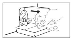
7. When no more water comes out, unscrew the pump cover by turning it anti-clockwise, using pliers, and remove the filter. Always keep a towel nearby to dry up any water spillage when removing the cover.
